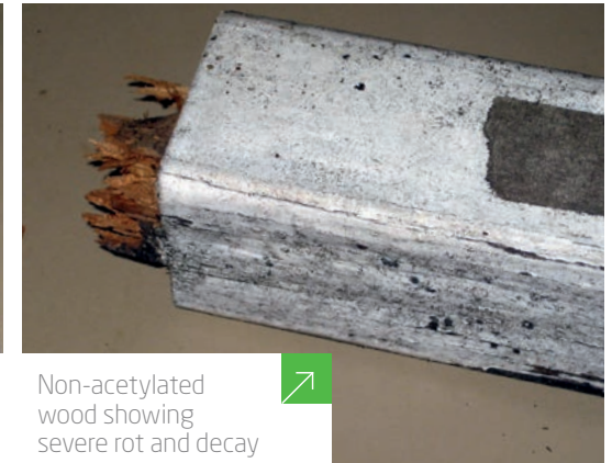
Non-acetylated wood showing rot and decay
