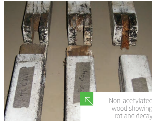
Non-acetylated wood showing severe rot and decay
