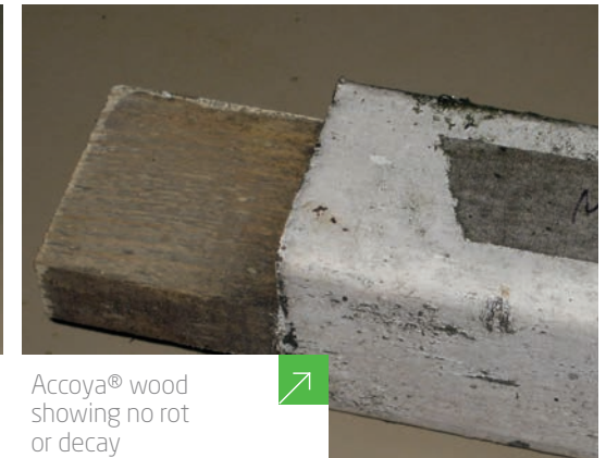
Non-acetylated wood showing severe rot and decay
